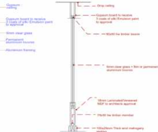
SECTION THROUGH FULL HEIGHT GYPSUM PARTITION WITH GLAZING
